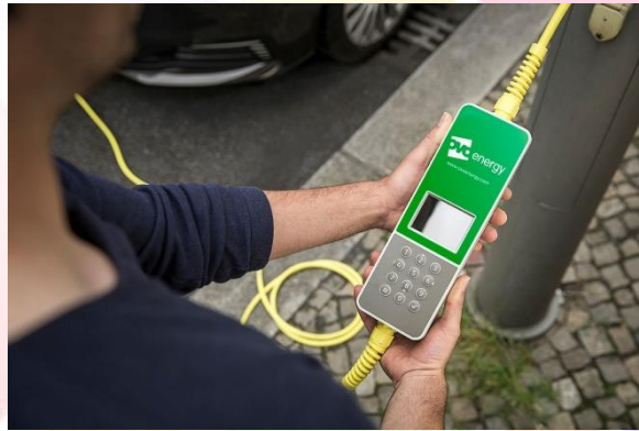
Fig.4. Smartmeter and cable [10]
