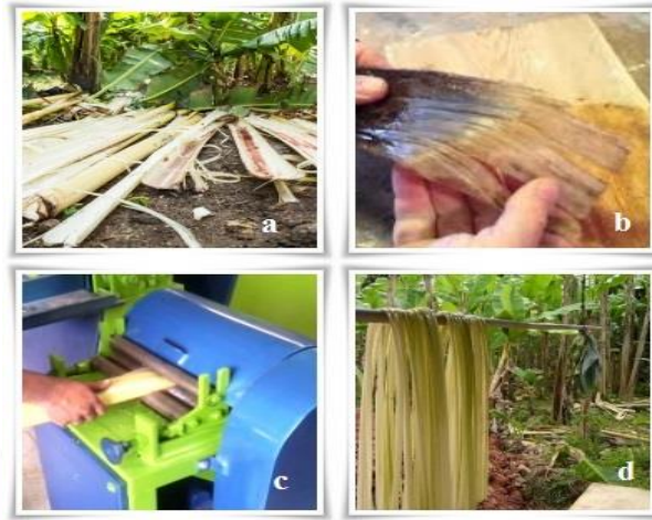
Figure 23: a) Harvesting of banana plant, b) Manual fiber extraction, c) Fiber extraction with decortication machine, d) Drying of banana fiber [40-43].
