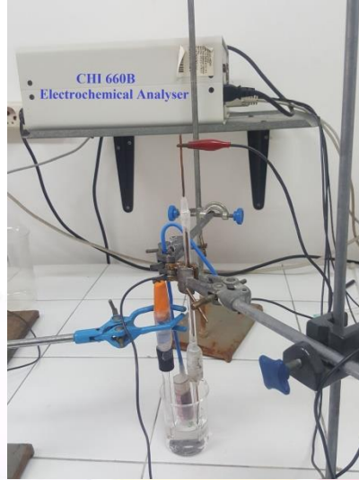
Figure 2: Three electrode cell experimental setup
