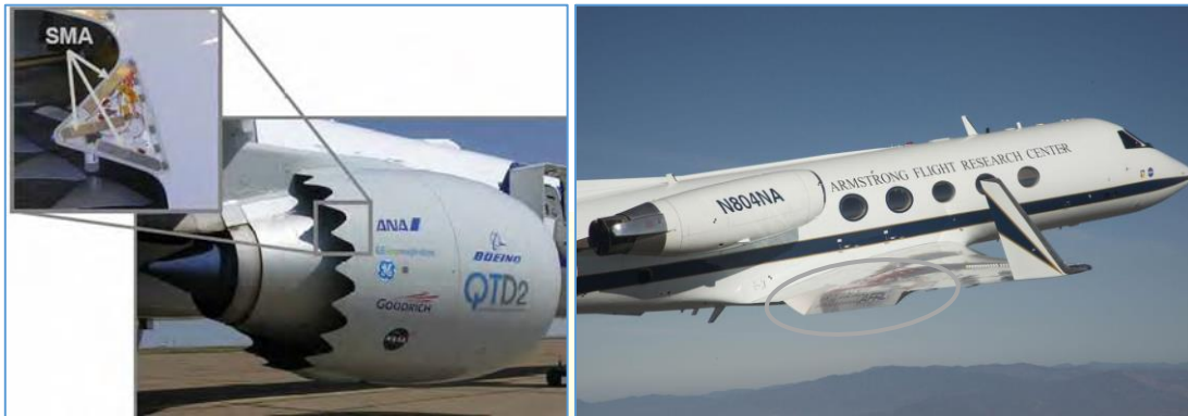
Figure 2: (a) BOEING, Variable Geometry Chevron (VGC); (b) NASA, Adaptive Compliant Trailing Edge (ACTE) project[3]
